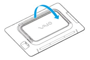
4. Pull up the top of the back panel (1), then remove it (2).
